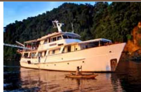
**Specifications:** 24 metre yacht, 5 x double/ twin air-conditioned cabins (3 with private bathroom), main saloon with TV, video, stereo, library, sundeck, small dive deck, camera tables, 2 x rigid hull inflatable's. Navigation Aids: VHF, HF, SSB radar, autopilot, GPS, satellite telephone.
